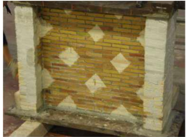
Fig 1. Wall surface with application of the two-component primer (Capozucca and Magagnini [10]).
