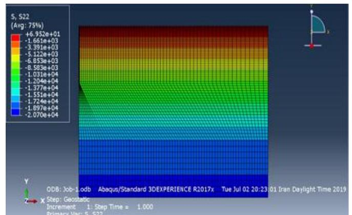
Fig 6. Meshing and stresses in Abaqus modeling.
