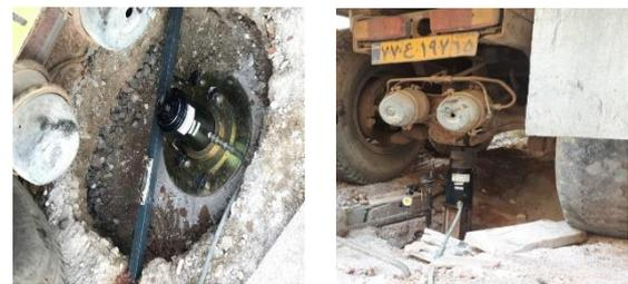
Fig 9. Loading plates during plate loading tests.
