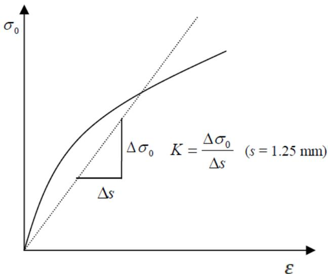
Fig 7. Definition of subgrade reaction modulus [14].
