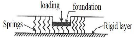
Fig 3. Schematic of the model provided by Winkler.
