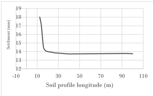
Fig 4. Results of model width subsidence in sensitivity analysis.
