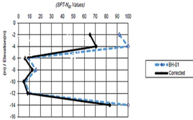
Fig 2. SPT changes in depth for samples extracted from the study area.
