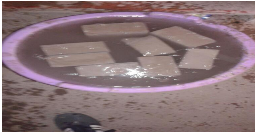
Figure 8. Lightweight concrete bricks mixes immersed in sulfate after 3 months
